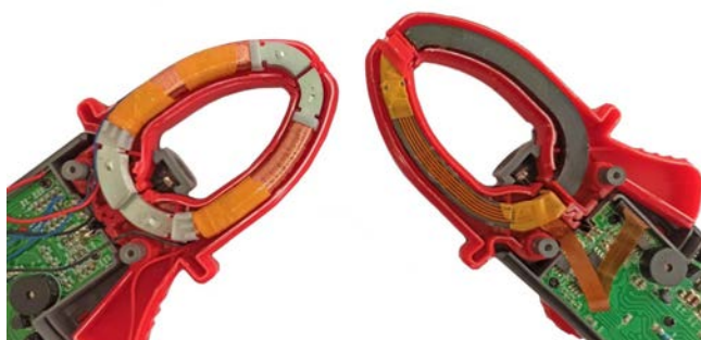
Figura 2. GAF-82C (transformador de corriente CA) vs GAF-82D (Efecto Hall CA/CC)
